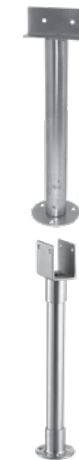
"L" TYPE PARTITION BRACE - Stainless Steel, Floor Mounted Unit supports 1/2" to 1-1/2" thick panels. Height is adjustable. Part No. 9A6005 - Adjusts 11-1/2" to 14" Part No. 9A85183 - Adjusts 9-1/2" to 12" Part No. 9A85193 - Adjusts 7-1/2" to 10"
