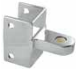
TOP HINGE 1-1/2" Bet. Screws For 1-1/4" Sq. Post Part No. 9CP400 A = 1-9/16"
