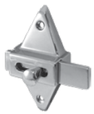
SLIDE BOLT ASSEMBLY 2-3/4" Bet. Screws 9/16" Bar to Door Clearance Part No. 9F0302 - Chrome Part No. 9F0302SS - Cast Stainless Steel
